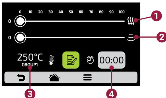
c) To change the Speed of Hot Air and Microwaves , just swipe the finger over the bar of each parameter or click on the desired location.
