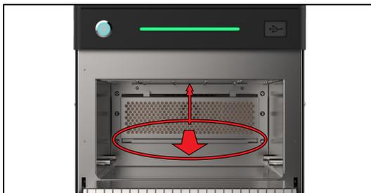
b) To sanitize it correctly, soak the catalytic converter in a bowl with warm water and neutral soap.
