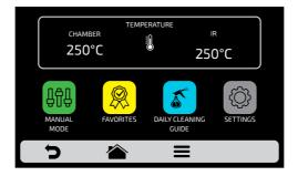
**c)** Set the parameters of Time, Temperature, Speed of Hot Air, Microwaves and bottom heating element (Infra-red).
