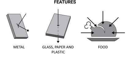
The use of plastic or paper material must respect it's specifications since it must support up to  $280^{\circ}$ C/  $536^{\circ}$ F and being microwavable.
