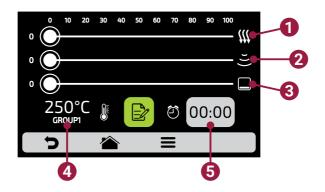
**c)** To change the impinged air speed, microwaves and bottom heating element wattage, just swipe the finger over the bar of each parameter or click on the desired location.
